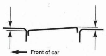
The sunroof is correctly adjusted when the edge toward the front of the car is level with, or 1mm below the roofline. The rear should be level with or 1mm above the roofline.
