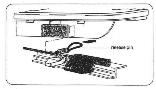
When the release pin is pulled, the rear guide is disengaged from the raising lever.
