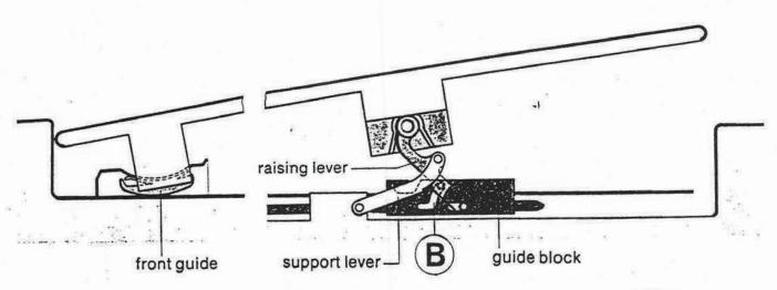
When the crank knob is turned the cables pull the guide blocks forward. The support lever lifts the raising lever and the front guide acts as a pivot. Recess (B) limits the opening angle.
