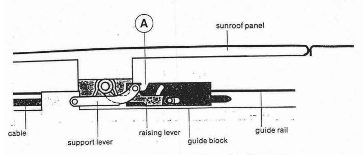
The support lever is attached to the body so that it can pivot. The raising lever connects the guide block to the sunroof panel. Recess (A) locks the sunroof panel in place when the roof is closed.
