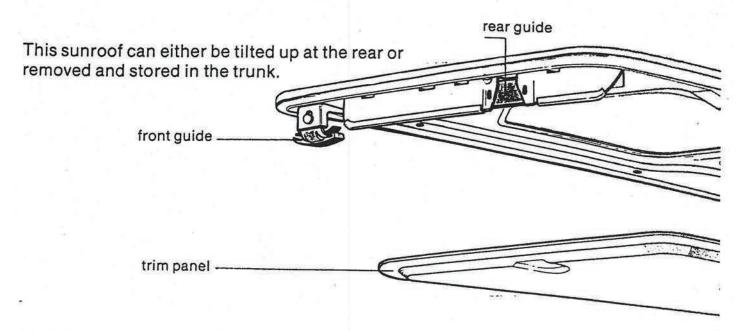
The frame assembly cannot be disassembled and is bolted to the body. The cables and tilting mechanism are part of the frame assembly.
