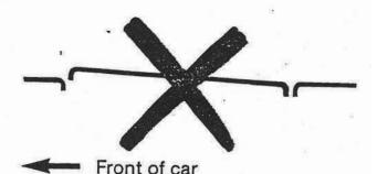
Sunroofs which are incorrectly adjusted can leak water and cause wind noise.
