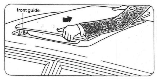
After the rear guide has has been disengaged, the sunroof can be lifted up and pulled back to release the front guides.
